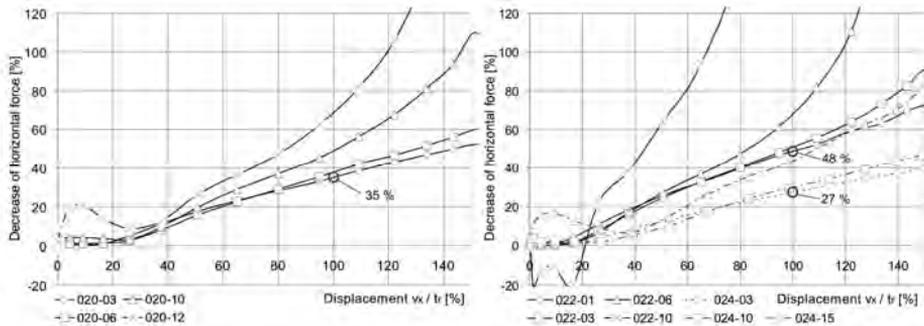
Fig. 1: Decrease of horizontal force of FREB due to rollout in comparison to SREB (fixed, without rollout) with (left) a height of 75 mm and (right, red) heights of 60 mm and (right, blue) 100 mm
