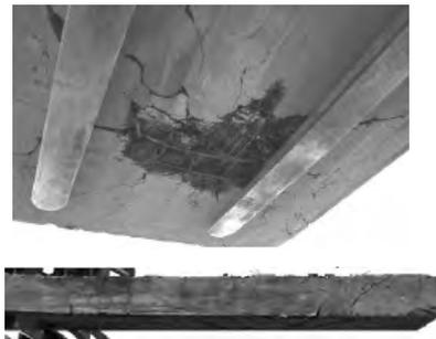
Figure 3: Fibre concrete panel after blast
