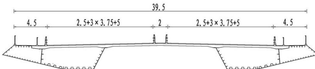
Fig. 2: Cross section of the composite box girder
