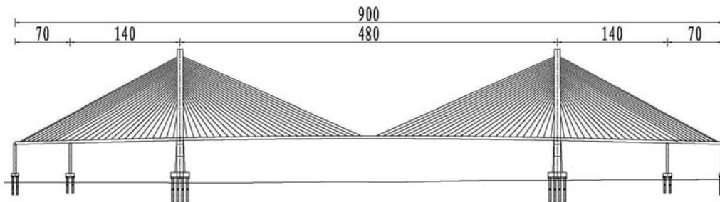
Fig. 1: Span arrangement of the second Jiaojiang Bridge
