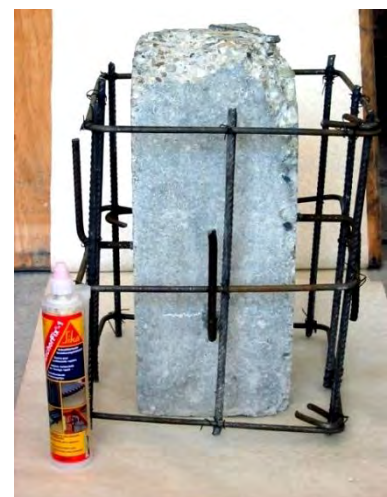
Fig. 1: RC columns strengthened by RC jacketing
